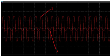
Figure 7. The oscilloscope display for the non-inverting operational amplifier
